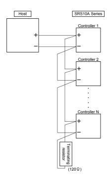
Note 1: With RS-485 specifications, you should mount the 1/2W 120Ω terminating resistor that comes with the termina element (between + and -) if necessary.
